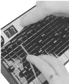
You can use the sliders on the **C16** to control volume, pan, effects sends, and many other parameters of many popular electronic musical devices (old and new). The **C16** is preprogrammed with the MIDI Control Change, MIDI Parameter and MIDI System Exclusive codes for manipulating the sound on a wide range of popular synths, sound modules, sound cards and software.
