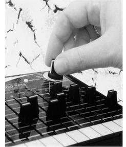
Target number 7 is called *Quick Mixer*, it provides easy access to volume, pan, reverb send, chorus send, variation effect send, balance and expression across sixteen MIDI channels simultaneously. The channel numbers correspond to the slider numbers. When this target is selected, the sixteen-position rotary control is used to change functions, so you can simply and rapidly switch between them.
