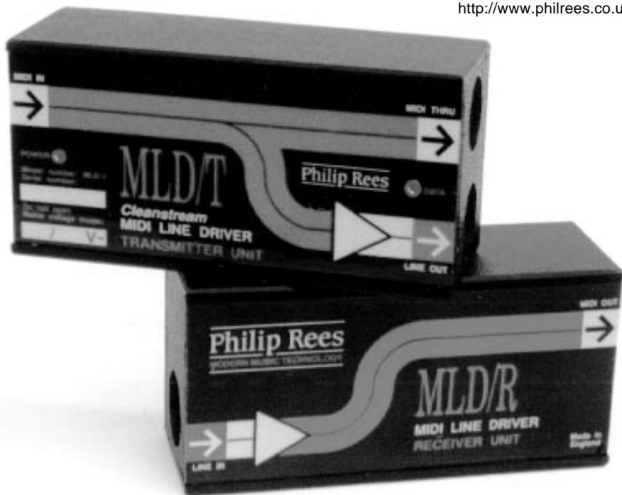
The **MLD** system overcomes the distance restriction (officially 15 metres maximum) of the standard MIDI hardware. It converts the MIDI signal to a differential (balanced) format and back again. This allows the signal to traverse up to a kilometre with quality screened twisted pair (STP) cable. Unscreened cable can also be used.
