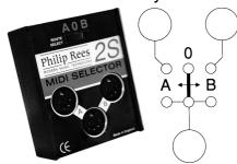
The high quality three position slide switch in the **2S** has three positions - marked 'A', 'O' and 'B'. In position 'A' the centre socket is connected to the left hand one. The centre position ('o') is the off position, in which none of the sockets is linked. Position 'B' links the centre and right hand sockets.
