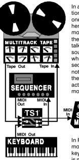
In an installation like the one shown here, BYPASS mode would let the keyboard talk to the sound module when the sequencer was not running; the **TS1** is not active in this mode.
